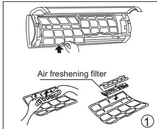
4. Remove the Air Freshening Filter from its support frame (on some models).
