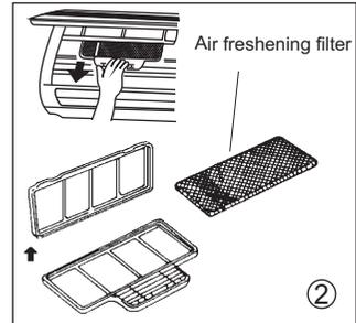
5. Install the air freshening filter back into position.
